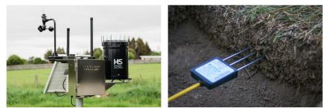
Photo 13 & 14 Harvest weather station and ground soil probe
